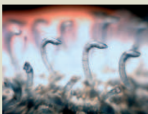
Above: Velcro hooks, magnified. Below: a shoe fastened with Velcro.
